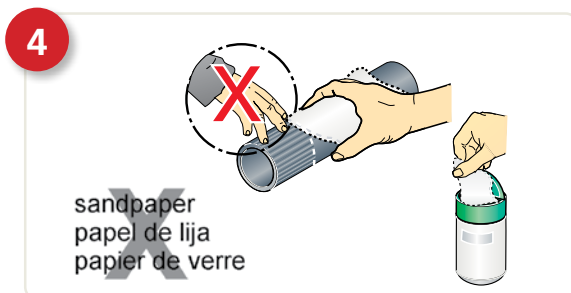
Clean with suitable degreasing agent
