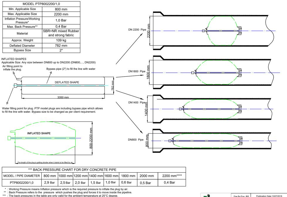
\*\*\*\* : It is not recommended to use the plugs in max. diameter except dry concrete pipe, because the back pressure is related with the friction coefficient between pipe and plug. If the pipe is not concrete or the pipe surface is not clean or not dry, the friction coefficient will be smaller. So, the Plug will hold less back pressure. So, don't use the plug in limits and select the larger size plug for that kind of applications.
