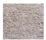
Gundseal® is a composite liner system consisting of sodium bentonite adhered to a polyethylene geomembrane. This acts as a barrier and provides the best leak protection for waste containment applications.
