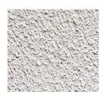
White Reflective helps to keep the liner cooler, resulting in fewer wrinkles. Fewer wrinkles mean the easier installation of cover soil and increasing the lifespan of the liner.
