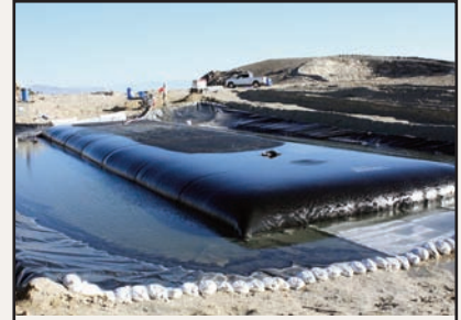
Gold mine tailings from barren and pregnant ponds dewatering in Geotube® containers.
