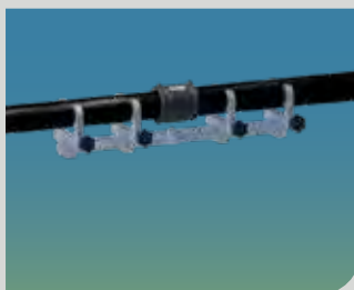
2. Example of clamping and alignment device
