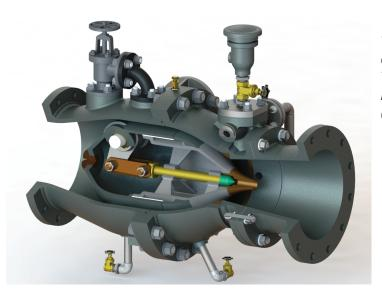
The Larner Johnson Valve is used for Free Discharge Control at pressure above that of the Fixed Cone valve. The valve can also be used for In-Line Pressure or Flow Control Applications and offers fine (full range) adjustment.
