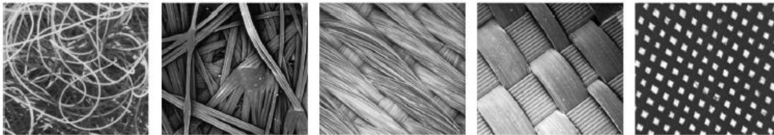
Figure 3. Types of geotextiles (a) needlepunched nonwoven (b) heatbonded nonwoven (c) woven multifilament (d) woven slit tape (e) woven monofilament (adapted from Bhatia and Smith 1996; Aydilek and Edil 2002)
