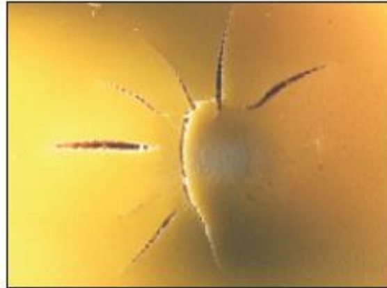
Fig. 10: Cracks in the inside wall of a PE 80 pipe subjected to an external point load and internal pressure (Test series 4)
